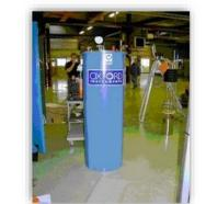
**Test Cryostats at Variable Temperature and High Magnetic Field (CETACEs)**
