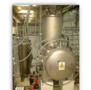
**Horizontal test Cryostat**
